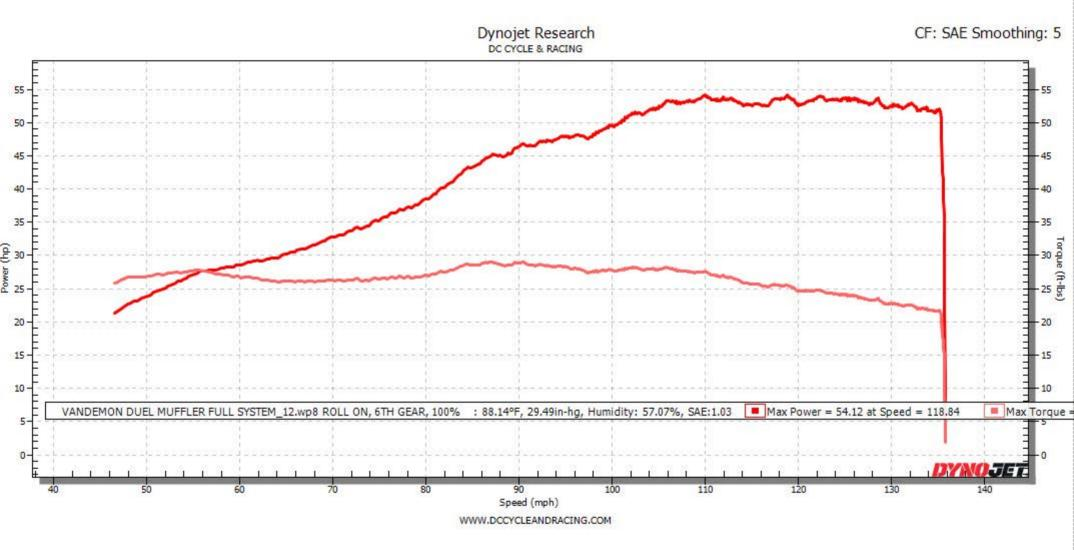
VANDEMON DUEL MUFFLER FULL SYSTEM\_12.wp8 [At: 5:26:34 PM, Wednesday, July 24, 2024] [Title: ROLL ON, 6TH GEAR, 100%] [As tested on Dynojet Model 250iX] [CF: SAE 1.03] [RPM: Inductive 1] [AFR Source: Dual WB2] Notes: VANDEMON FULL EXHAUST WITH DUEL CENTER MUFFLERS, DNA AIR FILTER AND LID, DC TUNE
